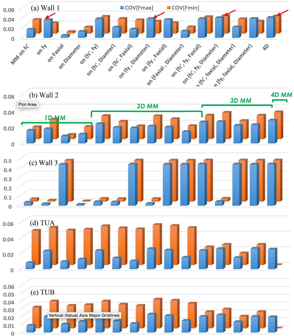
Figure 2.12. COV[F_{min}] and COV[F_{max}] obtained from 1D through 4D MM for (a) Wall 1; (b) Wall 2; (c) Wall 3; (d) TUA; (e) TUB. The variability of F_{axial} appears to govern the uncertainty of force-resisting capacity of Wall 3 while f_y appears to dominate the uncertainty of other four U-walls.
